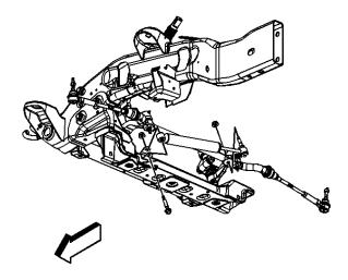
• Remove the shock absorber mounting bolt and the nut.
