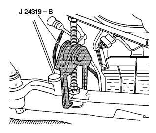
• Remove the shock absorber ball stud from the relay rod using the <u>J 24319-B</u> .
