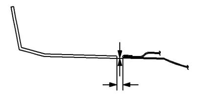
• Adjust the front door to fender gap to 5 mm (0.2 in).
