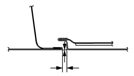
• Adjust the front door to rear door gap to 5 mm (0.2 in).
