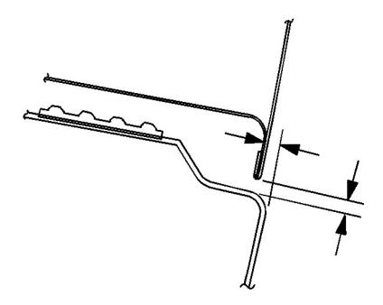
• Adjust the front door to rocker panel gap to 5 mm (0.2 in).
